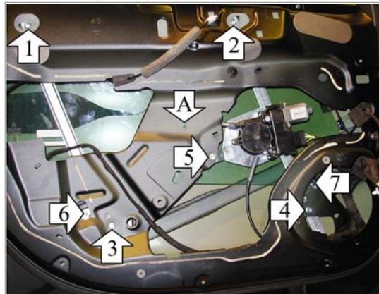
It is recommended not to remove the PVC gear clamp until mating with the engine in order to avoid possible unroll of the cable during assembly.
